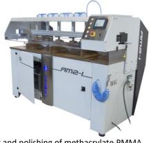
The AM2-i acrylic edge polisher has been designed for the machining and polishing of methacrylate PMMA workpieces.
